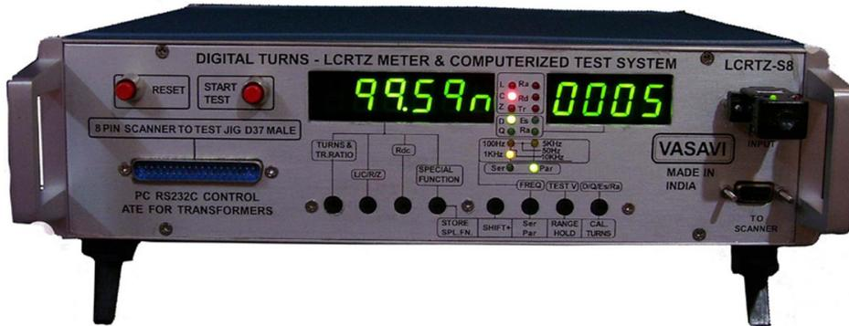
This Instrument is Specially designed for manufacturers and users of small transformers and coils like toroidal coils, Current Transformers, Bobbin Coils, SMPS Transformers, Pulse Transformers, Hybrid transformers, Potcore Transformers and RM-Core Transformers.
